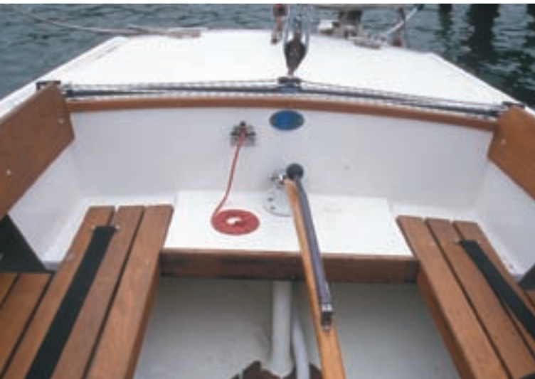
With the mainsheet led to a traveler aft of the cockpit, at left, a boom vang plays a vital role in shaping the mainsail. The companionway doors, at right, can be locked to secure items left in the cuddy.
